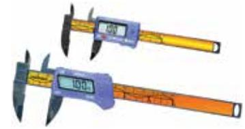
Available in 4 in. and 6 in. measuring ranges, these ergonomically designed calipers have an ultrasmooth slide bar that requires no lubrication. Units will run on the supplied battery for 10,000 hours. Resolution is 0.01 in. (0.1mm) and accuracy is ±0.01 in. (0.2mm). A serial-numbered certificate is provided from an ISO/IEC 17025 calibration laboratory indicating traceability N.I.S.T. standards.
