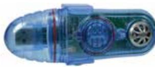
Back of CHD00408RH, Temperature and RH USB data logger
