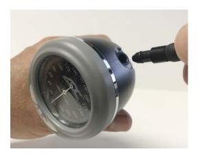
Slip-in style connection, not always clear when tube is fully inserted
