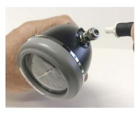
Bayonet connection "locks" in place when tube is fully mated
