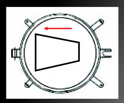
Thicker side of door gasket goes into the door groove
