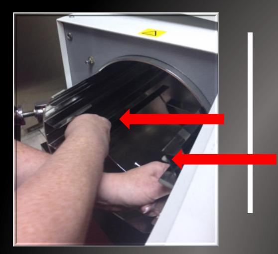
Step 2 Remove the tray rack from the autoclave
