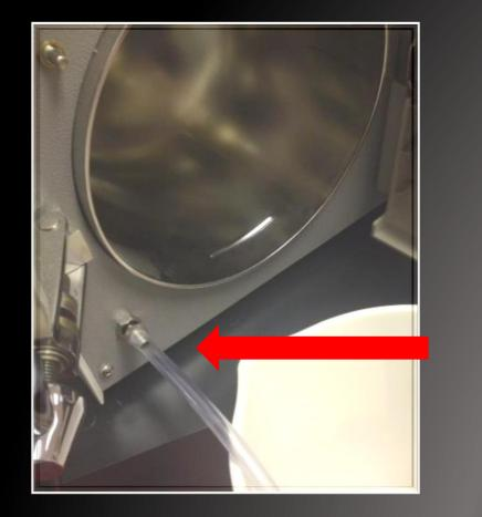
Step 9 (continued) Once the pressure gauge reaches "ZERO", open the chamber door and use the drain valve and drain hose to drain ALL of the water out of the water reservoir into a pail.
