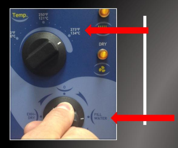
Step 9 *(continued)* Make sure the water reservoir is filled with steam distilled water.
