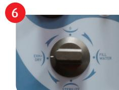
The pressure gauge will rise to 30psi and when the timer reaches "Zero" the bell will ring. Immediately turn the multivalve to "EXH+DRY" and the dirty water in the chamber will be forced out and back into the water reservoir
