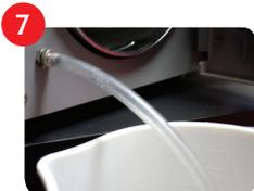
Once the pressure gauge reaches "ZERO", open the chamber door and use the drain valve and drain hose to drain ALL of the water out of the water reservoir into a pail. flush the reservoir with clean water. The Chamber Brite solution is in the waste water
