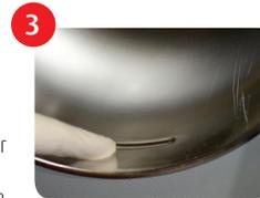
Water will begin to flow in from the back of the chamber. Monitor the flow until it gets to the indentation line at the front of the chamber.
