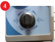
Turn the multivalve to "STERILIZE" (OLDER models are labeled "STE") Close and lock the door
