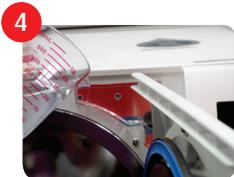
Refill the reservoir with clean steam distilled water. Note: EZ models top fill only EZPlus models top and front fill available
