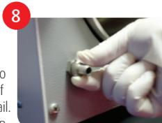
Tighten the drain valve. Refill the water reservoir with clean steam distilled water
