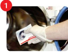
Cleaning needs to be done on a COLD chamber. Open the door and spread the ChamberBrite™ in a straight even line along the bottom of the chamber, from back to front. Do not leave a pile of Chamber Brite in one spot
