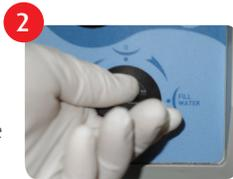
Make sure the water reservoir is filled with steam distilled water. Set temperature to 273°F (134°F). With the chamber door OPEN, turn the multivalve clockwise from "0" to "FILL WATER".
