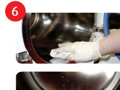
**TURN THE AUTOCLAVE OFF AND ALLOW THE CHAMBER TO COOL.** Once the chamber is cool, wipe the inside of the chamber and the water sensor at the rear with a damp cloth or sponge to remove any residue. Cleaning the dirt off the sides of the sensor is more important than the tip. The unit is now ready to sterilize.
