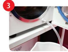
At the end of a cleaning cycle, open the chamber door and use the drain valve and drain hose to drain all of the water out of the reservoir into a pail. The Chamber Brite solution is in the waste water.
