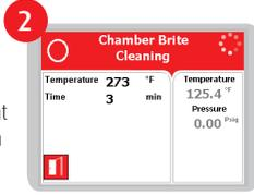
**EZPlus models:** Select Chamber Brite cleaning program, close the door and start the cycle.
