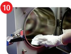
**TURN THE AUTOCLAVE OFF AND ALLOW THE CHAMBER TO COOL.** Once the chamber is cool, wipe the inside of the chamber with a damp cloth or sponge to remove any residue.
