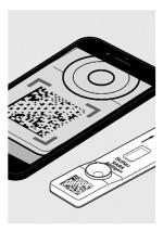
7. Follow App instructions to prepare the test cassette. Insert the prepared test cassette into the slot on the Sofia Q and the system will start automatically. In Walk Away mode, the test results will be displayed on the Sofia Q App screen in 15 minutes. In Read Now mode, the test results will be displayed on the Sofia Q App screen in about 1 minute. See the Sofia Q Interpretation of Results section.
