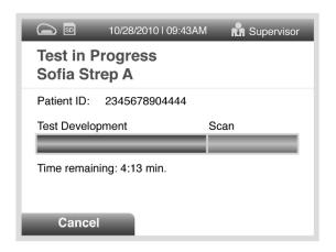
For example: This display shows that the test in WALK AWAY Mode has 4 minutes, 13 seconds remaining.
