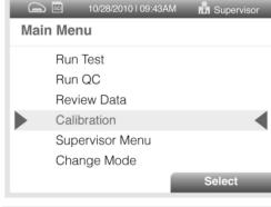
2. Following the prompts, insert the Calibration Cassette into Sofia and close the drawer. Sofia performs the Calibration Check automatically within two minutes with no user input required.
