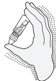
4. Remove the cap. Holding Bottle vertically, fill the Reagent Tube **to the line** [approximately 6 drops].
