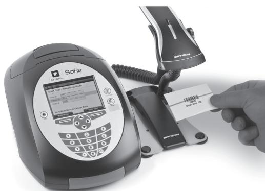
2. Input Patient ID and/or Order # using the handheld barcode scanner or manually enter the data using the key pad.
