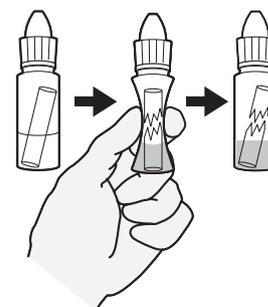
3. Vigorously shake the Bottle 5 times to mix the Solutions. Solution should turn green after the ampoule is broken.
