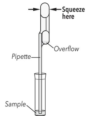
10. Firmly squeeze the top bulb to empty the contents of the Fixed Volume Pipette into the Cassette sample well. Extra liquid in the overflow bulb is OK.
