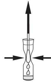
9. Fill the provided **Yellow 100  $\mu$ L Fixed Volume Pipette** with the sample:
