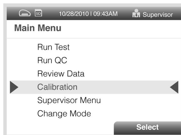
2. Following the prompts, insert the Calibration Cassette into Sofia and gently close the drawer. Sofia performs the Calibration Check automatically with no user input required.
