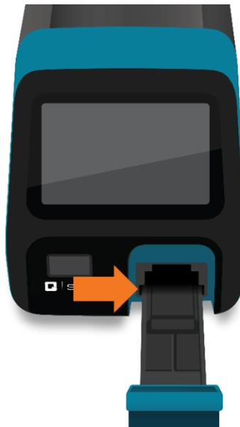
Gently slide the drawer until it is latched closed. If resistance is met or the drawer does not slide easily, check the alignment of the rails in the track. Go to the Main Menu and perform Calibration.
