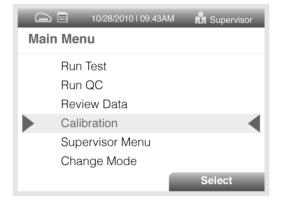
2. Following the prompts, insert the Calibration Cassette into Sofia and close the drawer. Sofia performs the Calibration Check automatically within two minutes with no user input required.
