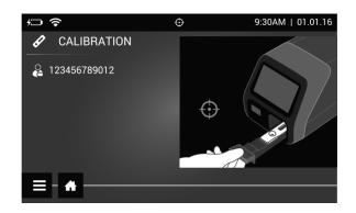
Sofia 2 indicates when the Calibration Check is completed. Select 👚 to return to the Run Test screen.
