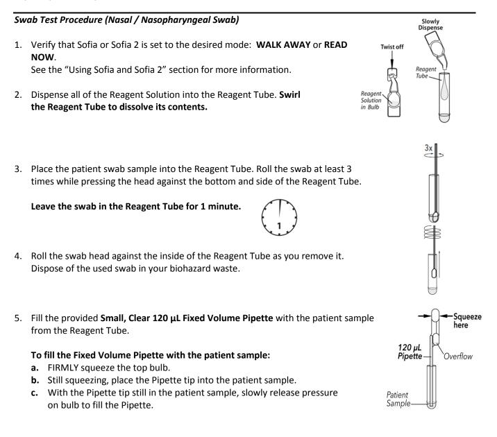
Firmly squeeze the top bulb to empty the contents of the Small, Clear 120 μL Fixed Volume Pipette into the Test Cassette sample well. Extra liquid left over in the overflow bulb should be left behind.
