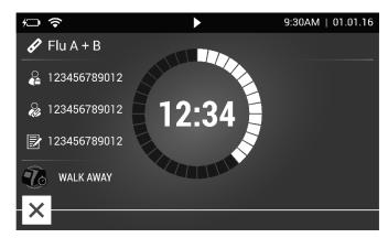
For example: This display shows that the test in WALK AWAY Mode has 12 minutes, 34 seconds remaining. Sofia 2 will read and display the results between 3 and 15 minutes.
