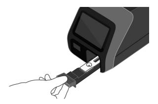
5. Sofia 2 will start automatically and display the progress, as shown in the example below. In WALK AWAY Mode, the test results will be displayed on the screen between 3 and 15 minutes. In READ NOW Mode, the test results will be displayed on the screen within 1 minute. See Sofia 2 Interpretation of Results section.
