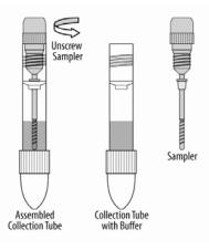
3. Randomly pierce the specimen with the grooved end of the Sampler in **at least five** (5) different sites.
