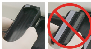
Figure 2-1: Urinalysis Strip Holder Position
