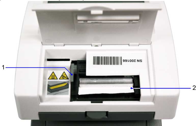
Figure 1-4: Printer Paper Compartment
