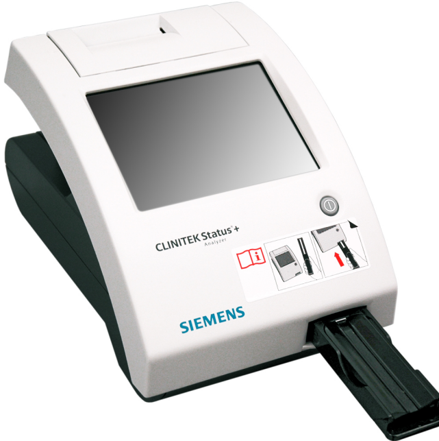
Figure 1-3: The Test Table and Test Table Insert
