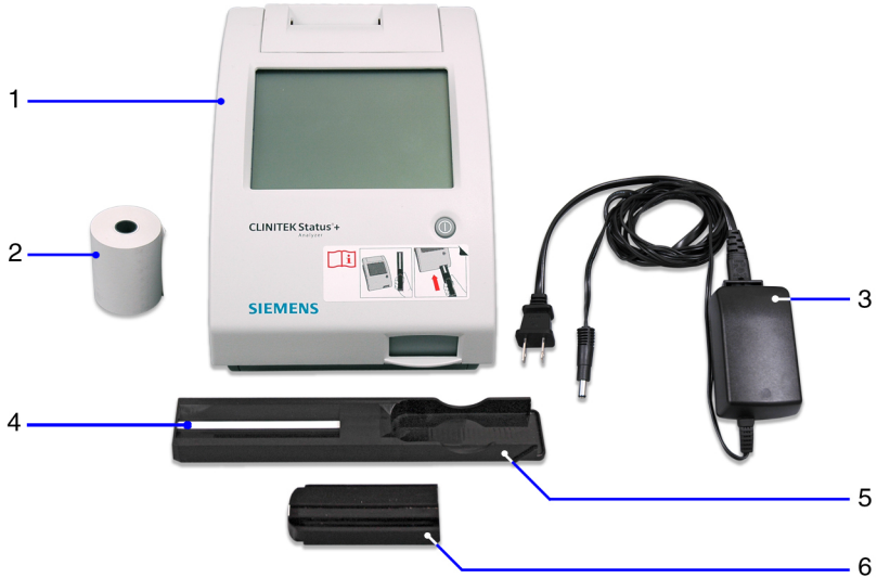
Figure 1-1: CLINITEK Status+ Analyzer Components
