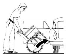
Lifting Wheelchair into Rear Seat or Trunk
